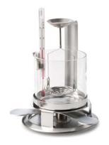
Density determination of solid and liquid samples is easy with this kit for analytical and precision balances.
